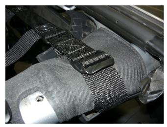
The next step is the rear corners. You need to take the long straps and feed them in between the roll bar and the sound bar. You may need to loosen of the sound bar bolts temporally so you can push the strap through. These bolts are found on the underside of the sound bar. Pull it through the bottom and up around the outside of the roll bar and connect to the ladderloc on the top again. Do this on both sides. Go around and adjust the net so the piece is centered on top.
