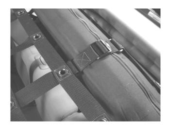
Install the two straps on the rear roll bar.
