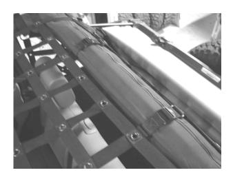
Install the front straps as shown. The straps get fed under the roll bar as shown (next page)
