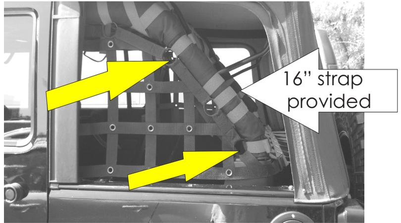
The remaining rings install using the 18" straps provided. These wrap around the top roll bar
