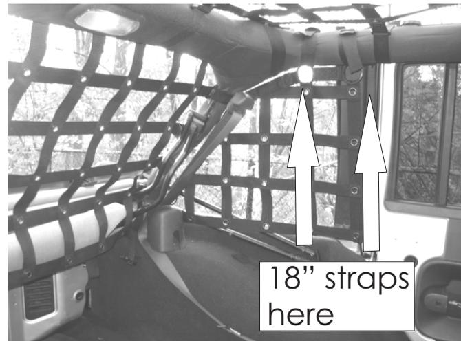
To install the bottom strap you need to pull back the carpeting from the rear quarter panel. Pass the webbing through the bracket as shown and connect into ladderloc on side net.
