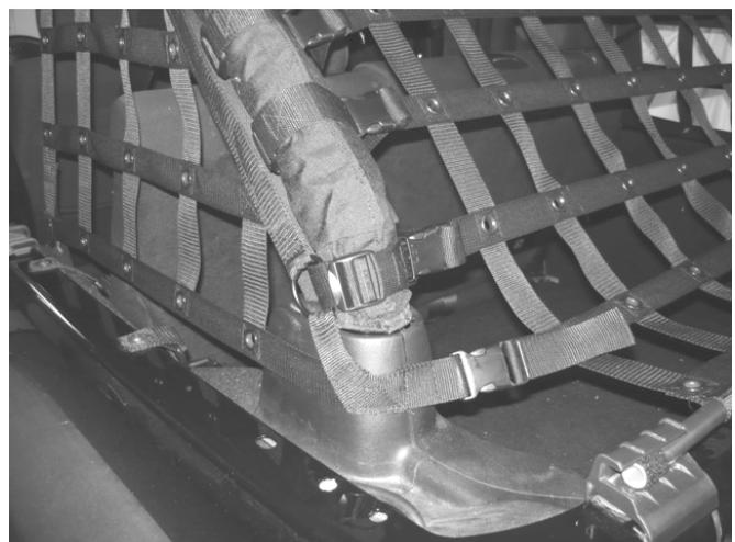
Slide each half of the tailgate bar in the last row as shown in the photo. This bar will connect at the center of the net and then the whole bar is clipped into soft-top tailgate clips. (Clips can be purchased from us or your local dealer.) This last row is optional and can be cut off if not needed.
