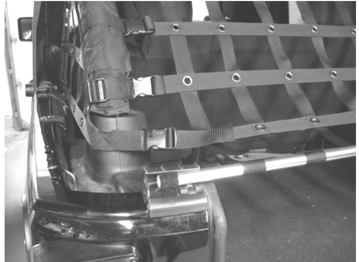
The strap at the very top of the rear piece wraps around the top of the vertical roll bar, comes toward the outside, wraps back around and connects into the ladderloc clip. See photo
