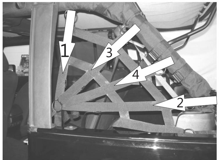
The last strap at the bottom can now be installed using the loop at the rear strap that you installed at the beginning.
