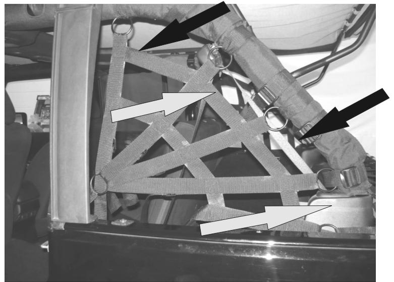
Next is to install is the attaching strap with the nut and washer provided. This is the strap that has a single ring on one end. This attaches to the existing bolt stud that you will find under the carpet directly behind the rear door
