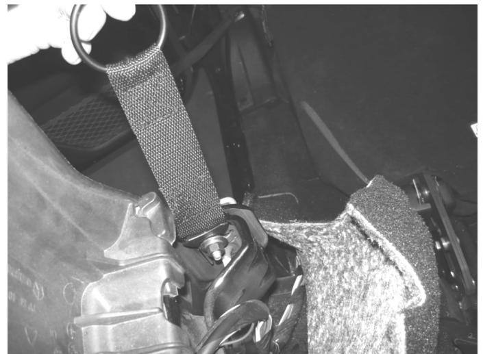
The side straps can now be installed on the loop in the order shown in the photo. Tighten straps 1 and 2 evenly so net is pulling equally in both directions. Followed by straps 3 and 4.
