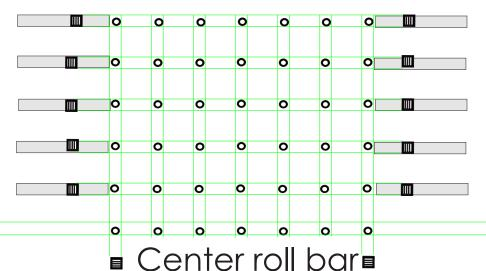
The last strap at the back wraps around the outside of the side roll bar at comes up around the center roll bar and connects to the ladderloc on the adjacent strap. See below
