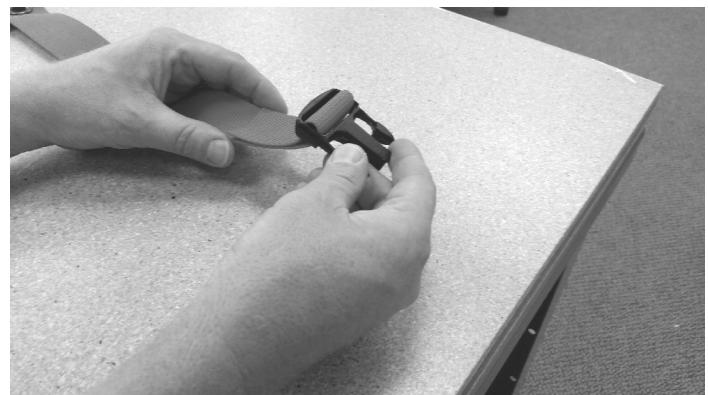
Start with the 2 top loops. Install 2 straps around the top roll bar. Use a tape measure to center or you can do this by eye and adjust later. Continue to do the 3 straps down each side. If you have the full netting system you will install the plastic buckles on the existing straps. Save the straps if you ever wish to install the pet divider without the rest of the netting system. Do not tighten the adjustment buckles at this time.
