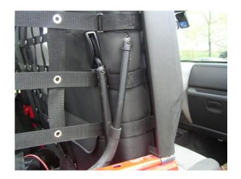
The next step is to install the back side. Start at the back and install the 8 buckles. Once all 8 are snapped in adjust the tension so the net is centered and evenly spaced.
