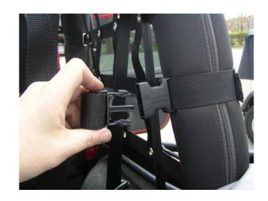
Continue with installing the balance of the straps along the top of your truck.
